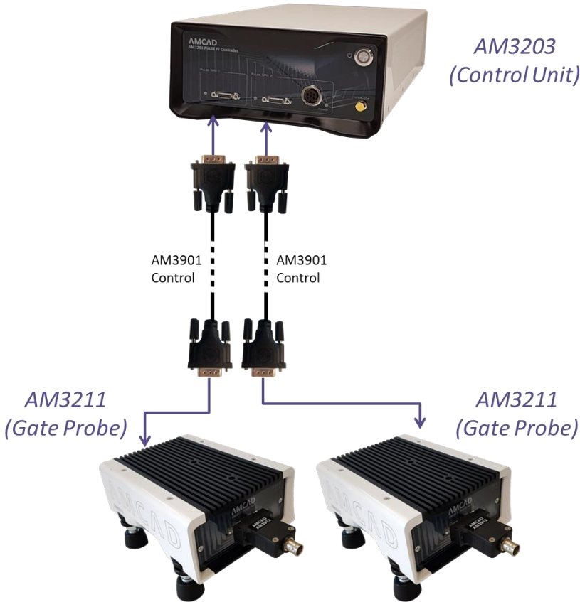
Figure 1:6 AM3200 configuration using 2 Gate pulser (AM3211)
