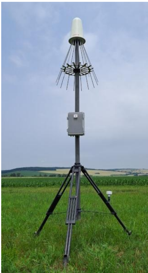
The WinRADIo WG-8800 VHF/UHF/SHF geolocation system utilizes the proven TDOA method (time-difference of arrival) with statistical signal processing.
