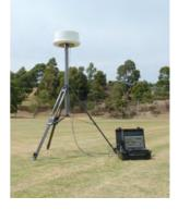
A high-performance integrated laptop computer is used for interfacing with the system and for processing and analyzing received signals.
