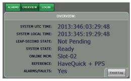
Available input reference selections include GPS (both C/A code and SAASM receivers are supported), IRIG-B, Have Quick/1PPS and external 10 MHz. In additional an MCM may be synchronized by up to 2 other MMC chassis using a fiber optic crosslink, this provides additional resiliency for the MMC time and frequency references.
