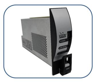
The *ViaLiteHD* HRC-5 rack card can be installed into the standard *ViaLiteHD* 19" rack shelf to monitor, log and raise alarms when events occur. The HRC-5 card utilizes SNMP protocol to communicate over Ethernet with the Horizons software package. If required, direct management of the HRC-5 is possible via a web browser, serial or CLI connections. The HRC-5 card gives control of RF over fiber and all other card types installed in the same 19" rack chassis.
