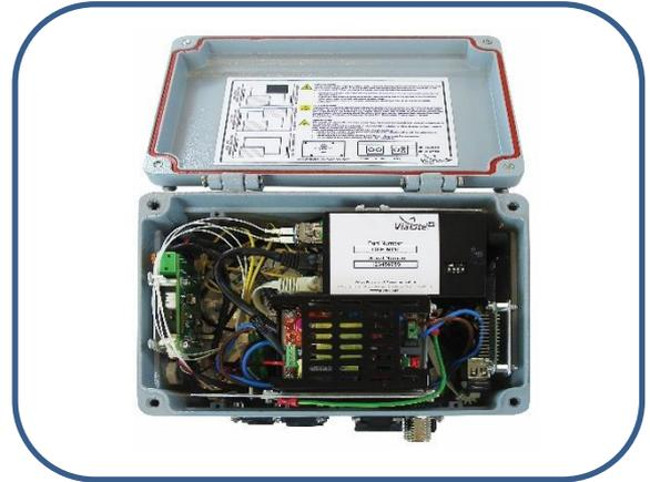
The *ViaLiteHD* ODE-MINI is a versatile enclosure designed for compact locations. The enclosure is cast aluminium and has an IP65 ingress protection rating. It is typically installed on a rooftop or antenna hub where RF and other services are transmitted over optical fiber to a remote equipment room. With options for fully integrated SNMP, Mini Ethernet Switch and LNA/B power, this enclosure is class leading for its size and cost.
