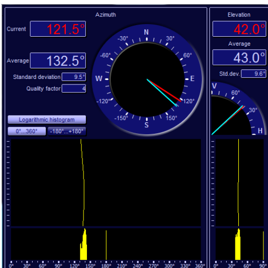
Example showing azimuth and elevation of sky wave on HF band
