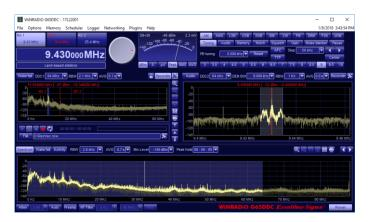
The receiver's superior performance results from its innovative, direct-sampling, digital down-conversion architecture along with the use of leading-edge components and design concepts. These all result in excellent sensitivity, selectivity and dynamic range, highly accurate and stable tuning, and perfect demodulation.
