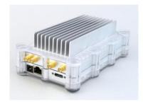
The receiver is very well shielded against interference, making it possible to operate in a noisy computer environment. Its modest power requirements are less than 12 watts. While connected via a LAN interface. thanks to PoE built-in functionality, the receiver can be operated and powered via a long Ethernet cable connection.
