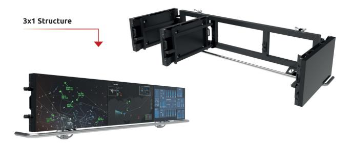
The MILCOTS's patented structure is qualified to resist shock and vibration inputs up to MIL S 901D inputs, and allows the system to pass the requirements of MIL STD 167. The folding and sliding shutter-system provides an easy access to each individual display of the wall, making installation and maintenance operations on the ship straightforward.
