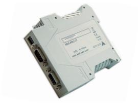
The MSX-RDC-17 is a device for supplying and acquiring a resolver. It converts the position value given by the resolver into a digital incremental output signal. The resolution of the incremental encoder output can be defined using the switch on the front side of the MSX-RDC-17.
