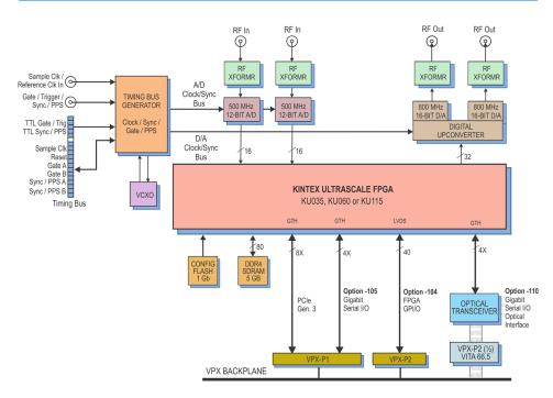
Standard front panel and VPX-P2 connections shown
