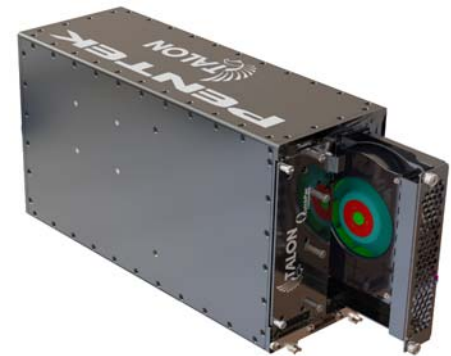
The fan assembly being removed from the back of the recorder
