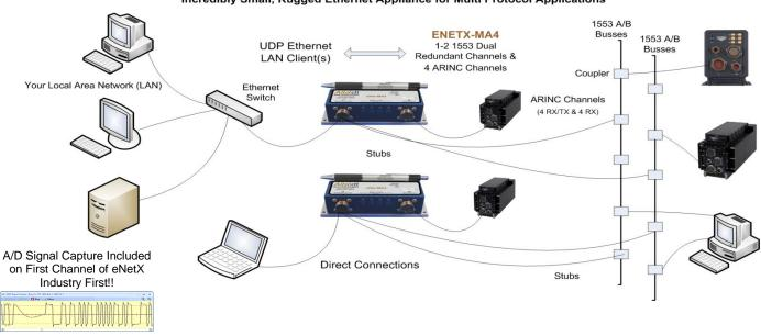
**eNetX-MA4**<sup>™</sup> is an innovative product for "remoting" 1553 & ARINC-429/717 operations on 10/100/1000 Ethernet local area networks (LAN). eNetX-MA4 is a very small, low-power, rugged device that provides real-time UDP connectivity to for 1-2 dual redundant 1553 (A/B) busses and 4 ARINC channels. Tested to MIL-STD-704F/810G/461F and DO160.
