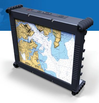
The RT10XG rugged portable panel is proposed with various configurations of Man Machine Interfaces. Lateral function keys and custom marking are proposed as an option, as well as high bright or NVIS to MIL STD 3009.
