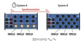
The combination of synchronisation and time stamp (TS) allows the clear allocation of signals that were captured by several systems.
