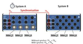
The combination of synchronisation and time stamp (TS) allows the clear allocation of signals that were captured by several systems.
