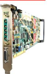
The BSM202 is capable of maintaining synchronization with the signal of interest to Eb/No of -3 dB when the signal transition density is 50%. When searching for the signal, acquisition is attainable in less than 50 bits. The unit is very robust and can maintain synchronization for a period of at least 256 bit periods without a transition.
