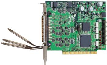
With the length measurement board APCI-3701, you can connect directly and acquire up to 16 half-bridge or LVDT transducers. The calibration software "ConfigTools" guides you through each step of the installation, beginning with the selection of a transducer from a database including more than 50 pre-calibrated transducers up to testing each single channel.
