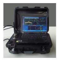
The WR-3300 unit is housed in a sturdy high-impact transport case containing one or two receivers with associated antenna interface circutry, power management system and a laptop. The built-in power management system allows operation from three sources: mains, vehicle battery or built-in rechargeable battery. The entire system is light-weight and easy to carry.
