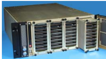
Figure 2. Chassis View showing one QuickPac canister partially withdrawn.
