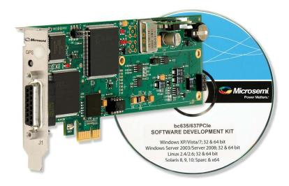
The Microsemi bc635PCle timing module provides unparalleled precise time and frequency functions to the host computer and peripheral data acquisition systems. Integration into a custom application is easy and efficient through the use of the full-featured standard Windows, Linux, and Solaris software development kits (SDKs)/drivers included with the module.
