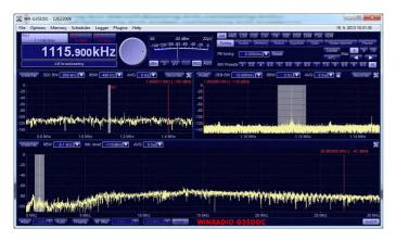
The receiver's superior performance results from its innovative, direct-sampling, digital down-conversion architecture along with the use of leading-edge components and design concepts. These all result in a very high IP3, wide dynamic range, high sensitivity, and accurate tuning. These key features create a receiver in a class of its own, with wide application potential, with many operational and instrumentation features not usually found on receivers of any price category.
