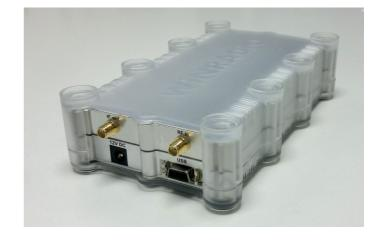
The WiNRADiO WR-G20DWC is a high-performance single-conversion frequency down-converter suitable for input frequencies up to 20 GHz.
