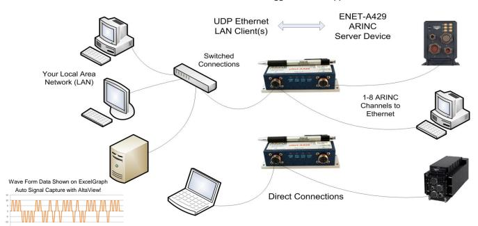
**eNet-A429**<sup>™</sup> is an innovative product that provides "remoting" of ARINC operations on 10/100/1000 Ethernet IP/UDP local area networks (LAN). eNet-429 is a small, low-power, rugged device that provides connectivity for 1-8 ARINC 429/575/573/717 Channels - Ideal for remoting ARINC connections for in-field applications or point-point lab usage.
