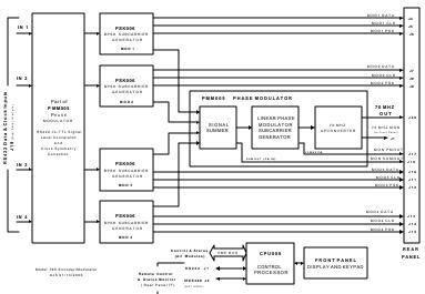
application to a Phase Modulator. The phase modulation can be turned OFF to provide a 12 MHz CW carrier. The phase modulated carrier is upconverted to 70 MHz. The output level of the 70 MHz IF PM carrier is programmable over a 20 dB range. The 70 MHz output is connected to the rear panel interface. A sample of the 70 MHz output as well as the summed subcarriers are provided as outputs for connection to test points.
