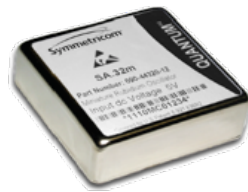
Figure 12: Rubidium miniature atomic clock, embedded component in timing equipment.
