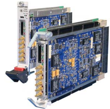
Model 52650 3U VPX COTS and rugged
