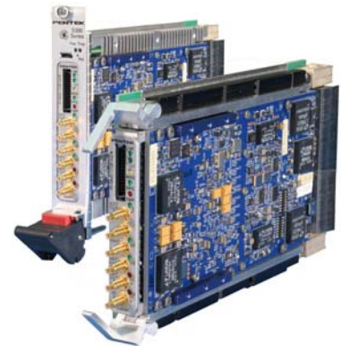
Model 53690 3U VPX COTS and rugged
